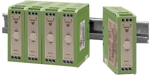
Transducer output is derived from the average absolute value of the input and calibrated as the RMS value of a sine wave input.
